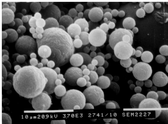
Figure 34. Methylpyrrolidinone chitosan microspheres obtained by spray drying.
